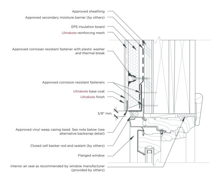
NOTE: Maintain 1/8" space between beveled insulation and weep casing bead.
